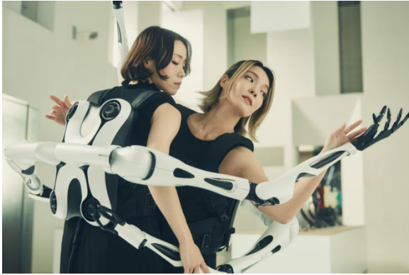
Jizai Arm, an artificial limb that co-create choreographic dance responding to the performer. Image source: https://newatlas.com/robotics/jizai-arms-supernumerary-robotic-arm-system/
